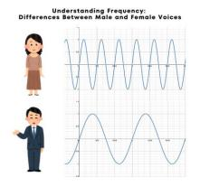
Note. Displaying the sound graphs of male and female voices as a real-life example helps illustrate the concept of frequency. Frequency is one of the key factors in sound graph analysis, playing a crucial role in understanding variations in pitch and tone.
