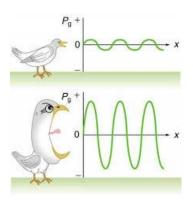
Note. Adapted to illustrate intensity as a key factor in sound graphs and demonstrate the qualitative representation of high and low intensity. Adapted from "17.3: Sound Intensity and Sound Level," Lumen Learning, n.d. (https://courses.lumenlearning.com/suny-physics/chapter/17-3-sound-intensity-and-sound-level/)
